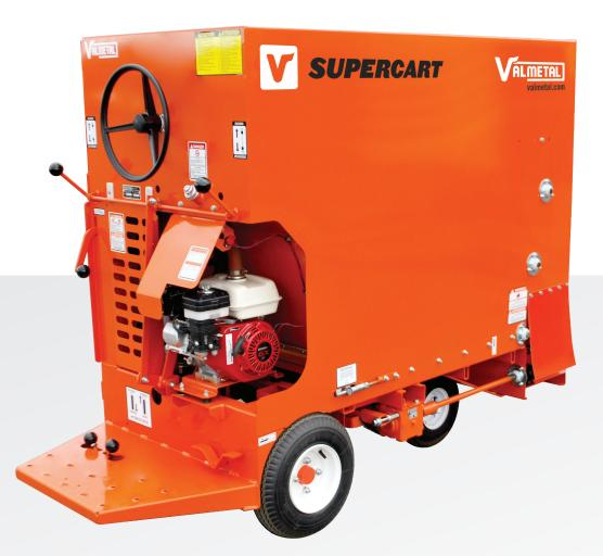
The CC model features a cross conveyor driven by a sturdy reversible gearbox that allows unloading on either side of the cart for more flexibility. Foot operated, all the components are underneath the cart to eliminate damage from curbs and doorways.
