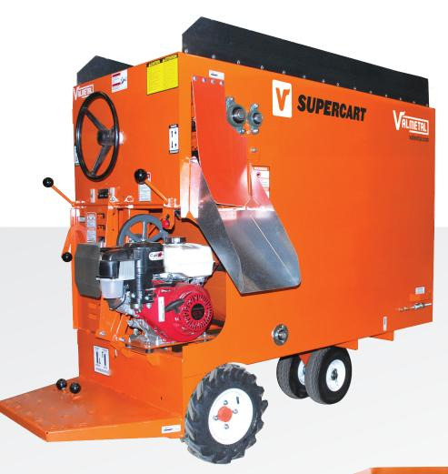
Specially designed for elevated mangers, the HT model features an inclined bottom section and twin discharge augers to evenly discharge the ration (right side only). A 16" long slide is supplied with the cart to carry the feed further away if needed. The bottom of the discharge opening is 40" from the floor.
